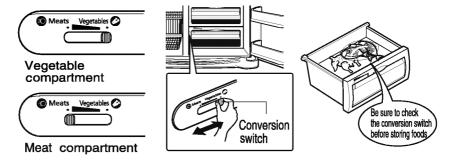
The meat compartment maintains the temperature at a lower point than the refrigerator compartment so that meat or fish can be stored fresh longer.
