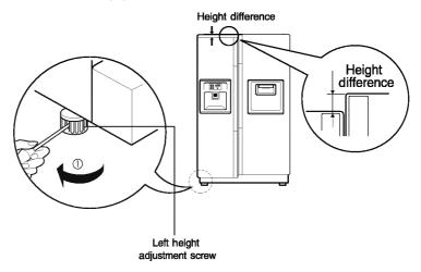
If the freezer compartment door is higher than the refrigerator compartment door Level the door by inserting flat (-type) driver into the groove of the right height adjusting screw and rotate it clockwise (①).
