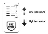
Generally, 3 (Normal) is correct for food storing. Select an appropriate setting 1 (Warmest), 2 or 4, and 5 (Coldest) according to the storage amount and frequency of use.
