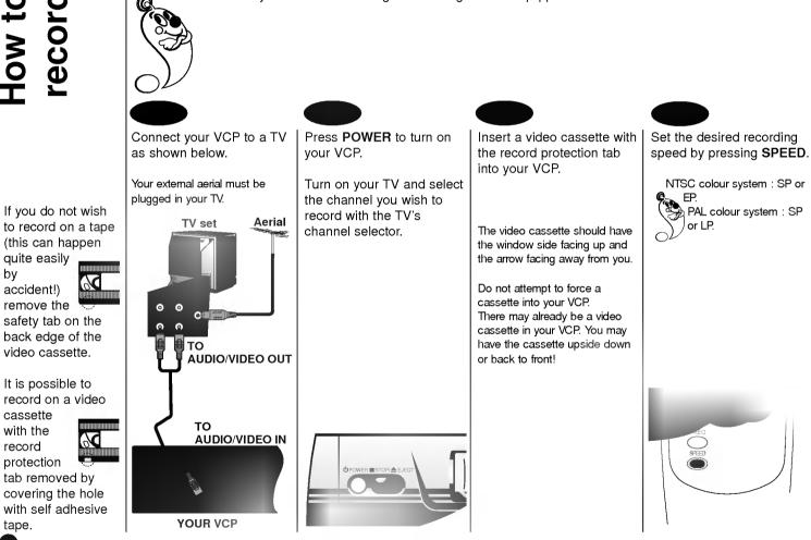
Your VCP allows you to make recordings connecting to a TV equipped with AUDIO and VIDEO sockets.
