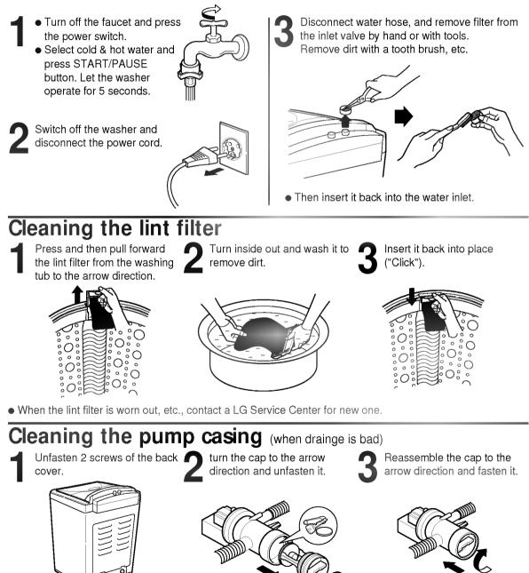
• CAUTION : Check it over if water leaks after reassembling.(Rubber ring is in the cap)
