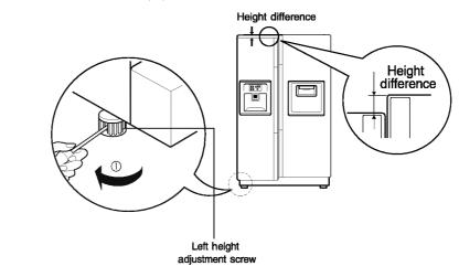
If the freezer compartment door is higher than the refrigerator compartment door Level the door by inserting flat ( - type) driver into the groove of the right height adjusting screw and rotate it clockwise  $(\mathbb{O})$ .
