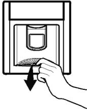
2 Dispose of the water in the kitchen sink, wash the drip tray and the grille with a mild detergent and rinse thoroughly.
