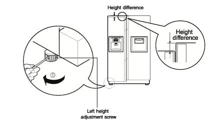
Level the door by inserting flat ( – type) driver into the groove of the right height adjusting screw and rotate it clockwise ( $\mathbb{O}$ ).
