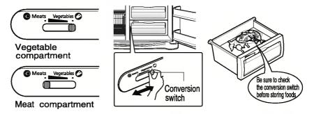
The meat compartment maintains the temperature at a lower point than the refrigerator compartment so that meat or fish can be stored fresh longer.
