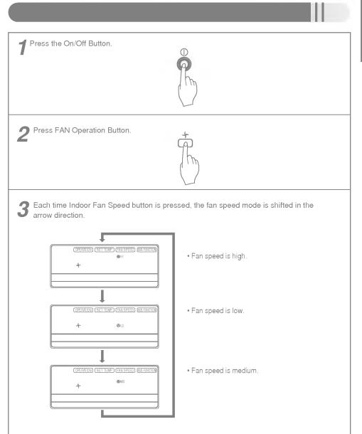
\* You can't set the temperature in Fan Operation mode. To exit this mode, press 'Operation Mode' button.
