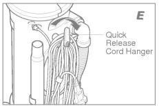
To release the cord, rotate the quick-release cord hanger downward. (Fig. E)
