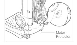
The motor protector by-pass valve may open when using attachments or when cleaning new carpet, due to reduced air flow caused by the attachments themselves or by new carpet reduce filling the dust container quickly.
