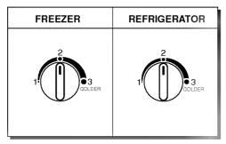
Initially, set the freezer and/or refrigerator compartment control at "2"(mid position).
