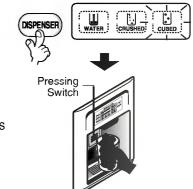
Reference: Please wait for 2-3 seconds in order to take final ice slices or drops of water when taking out cup from the pressing switches after taking ice or water.
