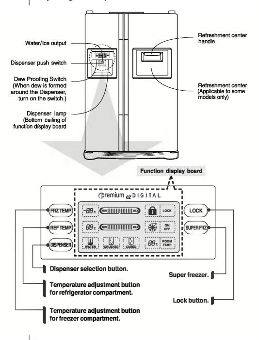
You can adjust temperature of and freezer room and refrigerator room.
