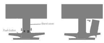
2. After connecting cables, put the **stand cover** correctly into the holes on the stand. If securely connected, you can hear the click sound from the latch.
