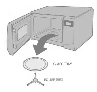
Flace the oven in the level location of your choice with more than 85cm height but make sure there is at least 30cm of space on the top and 10cm at the rear for proper ventilation. The front of the oven should be at least 8cm from the edge of the surface to prevent tipping.
