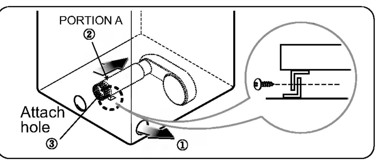
$\mathbf{3}$ . Reconnect the new duct[11 in(28cm)] to the blower housing, and Fixing the duct to the base.
