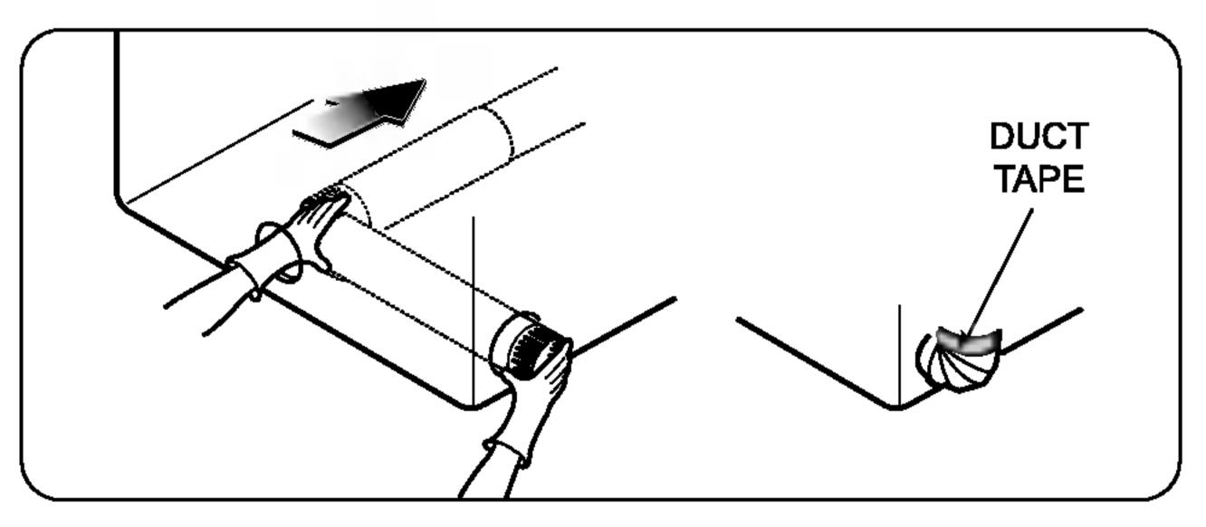
**5.** Insert duct assembly, elbow first, through the
