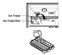
To remove ice cubes, hold the knob of the tray and turn gently. Then, ice cubes drop in the ice cube box.
