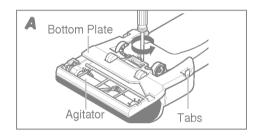
Pushing the locking tabs toward the center of the vacuum, pull the bottom plate away from the nozzle housing. (Fig. B)
