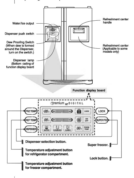
You can adjust temperature of and freezer room and refrigerator room.
