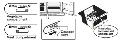
The meat compartment maintains the temperature at a lower point than the refrigerator compartment so that meat or fish can be stored fresh longer.
