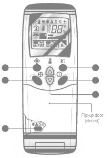
START/STOP BUTTON Operation starts when this button is pressed and stops when the button is pressed again.
