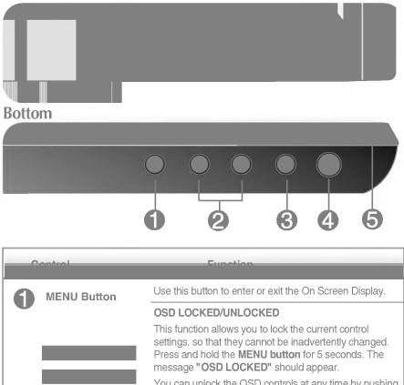
You can unlock the OSD controls at any time by pushing the **MENU button** for 5 seconds. The message **"OSD UNLOCKED"** should appear. Use these buttons to select or adjust functions in the On
