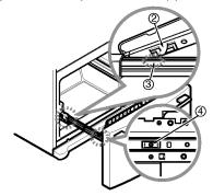
With the drawer pulled out to full extension, insert the lower basket (5) in the rail assembly until it doesn't move forward.
