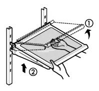
To replace a shelf—Tilt the front of the shelf up and guide the shelf hooks into the slots at a desired height. Then lower the front of the shelf so that the hooks drop into the slots.
