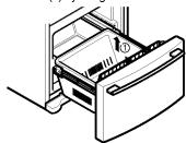
Remove the screw (2) from each side of rail system.
