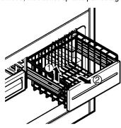
To Install, pull both rails out to full extension. Hook the basket supports into the rail tabs and push to the back of compartment.
