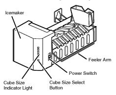
The icemaker will produce eight cubes per cycle—approximately 100–130 cubes in a 24-hour period, depending on freezer compartment temperature, room temperature, number of door openings and other operating conditions.
