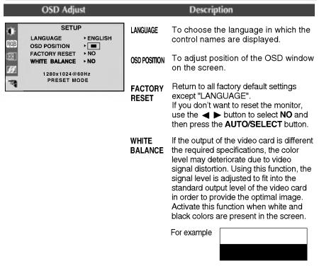
If this does not improve the screen image, restore the factory default settings. If necessary, perform the white balance function again. This function will be enabled only when the input signal is an analog signal.
