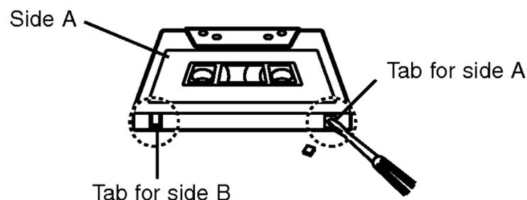
To record again, cover the hole of the tab with adhesive tape.
