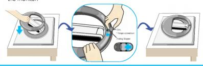
■ Tighten the four **5** screws about half into the slots in the base part, hold the two screws at the bottom to pull them inward, and then tighten the screws all the way.
