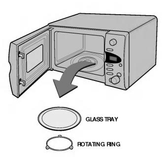
Place the oven in the level location of your choice with more than 85cm height but make sure there is at least 30cm of space on the top and 10cm at the rear for proper
