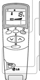
Open the door on the remote control. Press the PLASMA air purifying operation ON/OFF button. Operation will start when the button is pressed and stop when the button is pressed again.
