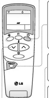
Open the door on the remote control. To select Healthy Dehumidification Operation, press the Operation Mode Selection button.
