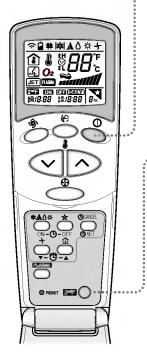
Open the door of the remote control and press the 2nd Function button to operate functions printed in blue at bottom of buttons.
