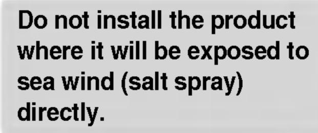
It may cause corrosion on the product. Corrosion, particularly on the condenser and evaporator fins, could cause product malfunction or inefficient operation.
