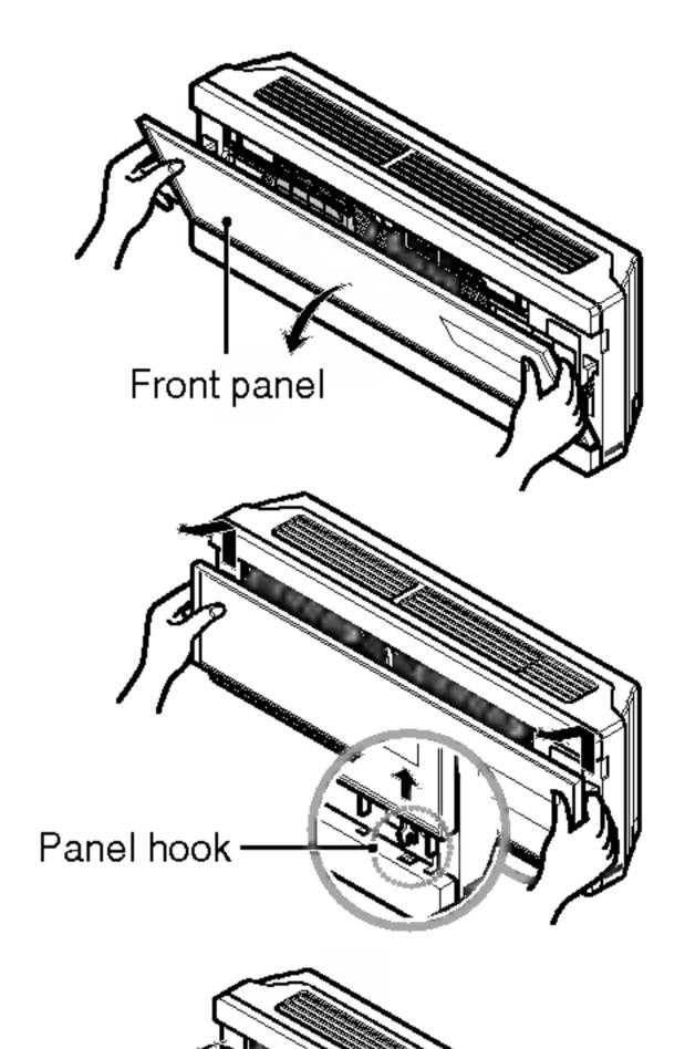
3. Come down the panel and then remove the air filter.
