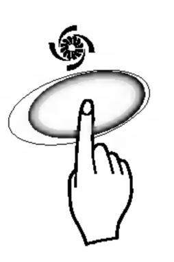
To cancel the **Jet Cool** mode, press the **Jet Cool** button, the fan speed button or the room temperature setting button again and the unit will operate at high fan speed on cooling mode.
