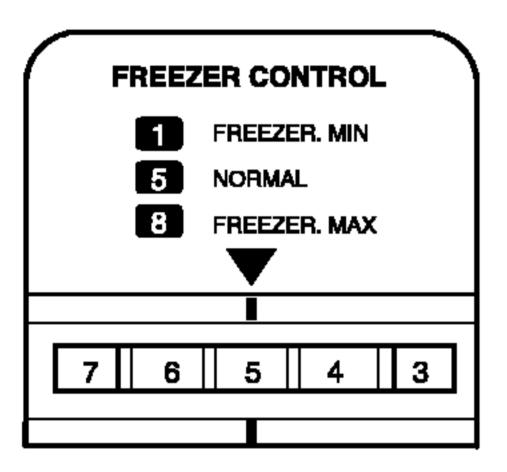
• FREEZER CONTROL - 1, 2, 3, 4, 5, 6, 7, 8 Setting at "8", the freezer compartment becomes colder. But the refrigerator compartment becomes warmer because less cold air flows into the refrigerator compartment.
