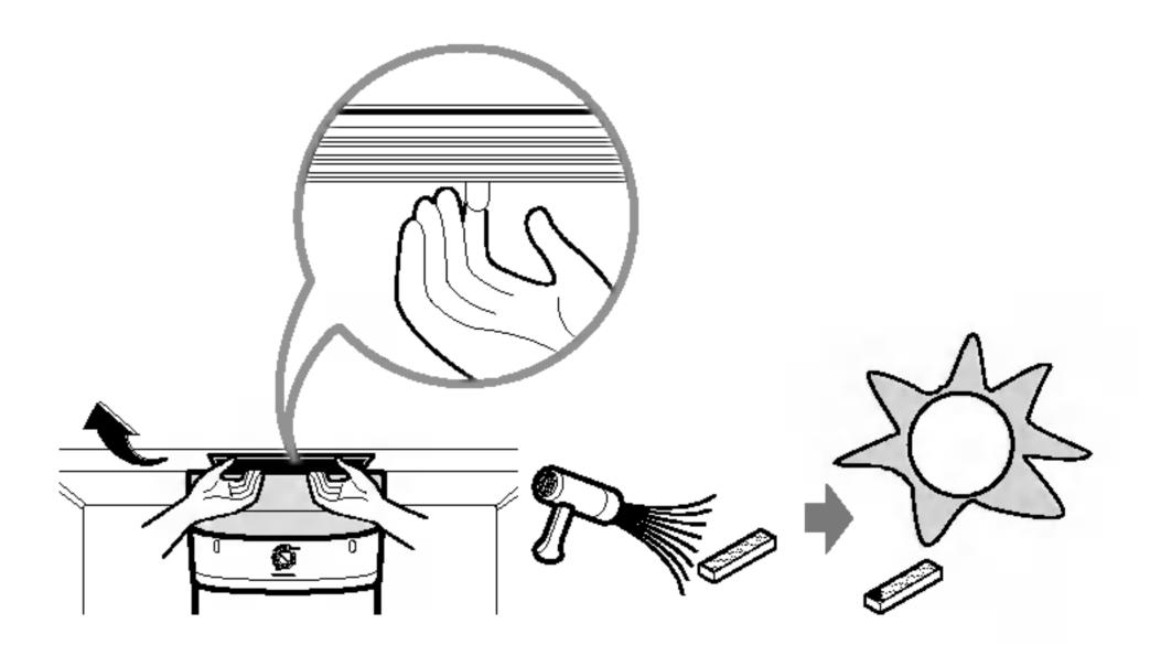
Separate deodorizer in ceiling of refrigerator compartment, using hair drier to remove moisture or malodor and oxidize under sunlight to decomposing malodor by ultraviolet.
