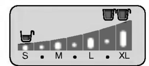
• When the water level is automatically detected, it may differ depending on the quantity of laundry even though the same water level is indicated on the control panel.
