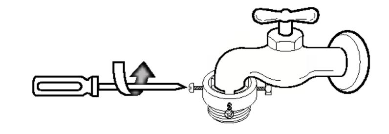
Attach the water supply hose ensuring it connects securely to the connector or the water tap
