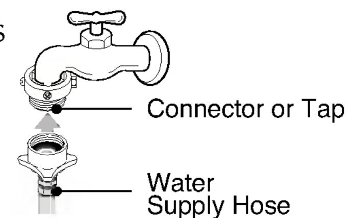
Tighten the connection between the water supply hose
