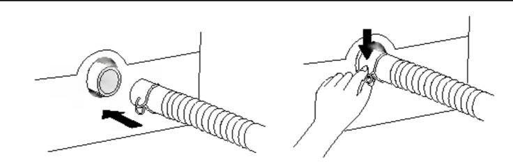
Put the other end of the drain hose over the standpipe or wash tub.
