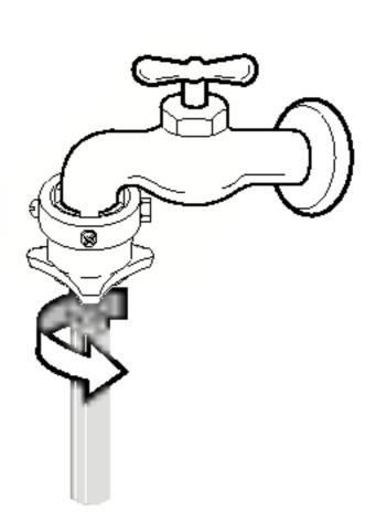
Check the connection of water supply hose and the connector
