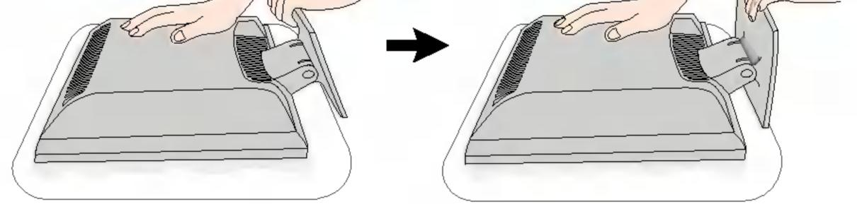
Place the monitor upright and adjust the angle of the stand base as desired.
