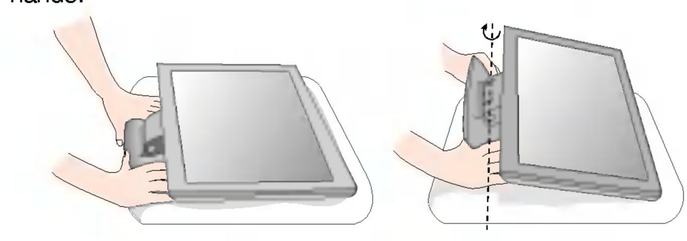
2. Place the monitor with its front facing downward and then further expand the stand base fully to 90 degrees. Do not apply excessive force to expand the stand base over 90 degrees as it may damage the monitor.
