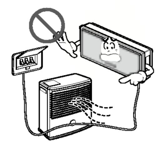
Do not allow water to run into electric parts.
