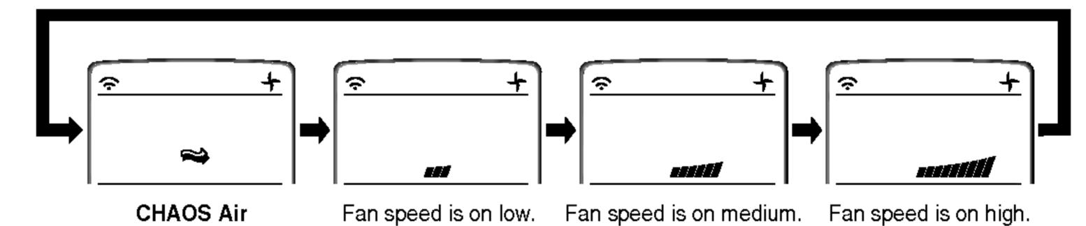
CHAOS Air economizes power consumption and prevents overcooling. The fan speed is automatically changed from high to low or vice versa, depending on the ambient temperature.
