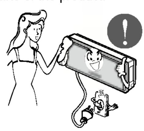
Do not touch the metal parts of the product when removing the air filter. They are very sharp!
