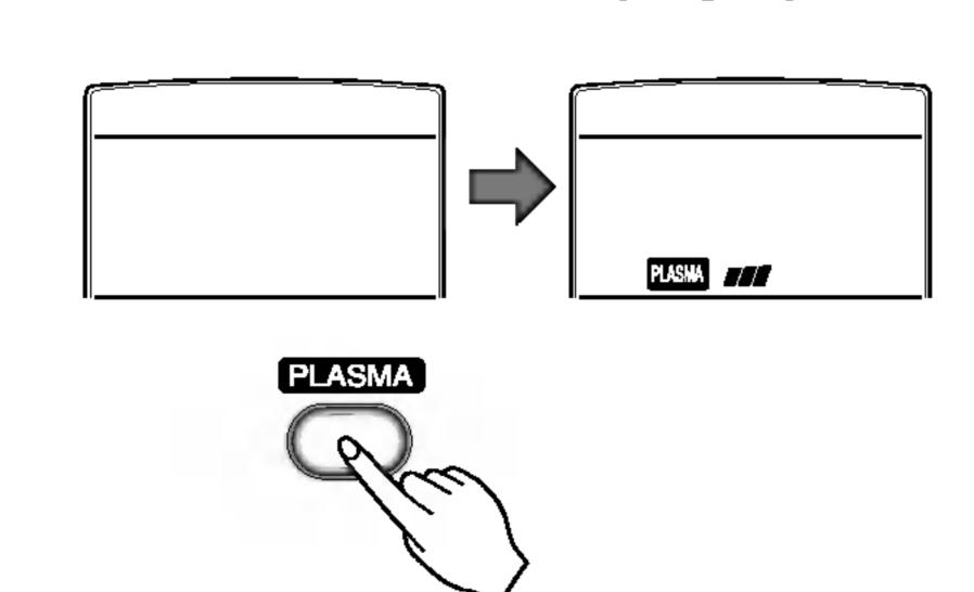
If you press the only PLASMA button, only PLASMA purification function operates. Then, fan speed is low. You can select the fan speed in four steps-low, medium, high or CHAOS.
