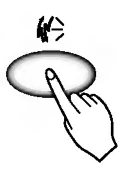
Press the button again and the louvers will stop. After 30 minutes, the louvers return to the maximum airflow position automatically.
