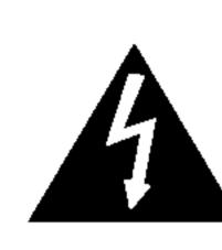
The lightning flash with arrowhead symbol, within an equilateral triangle is intended to alert the user to the presence of uninsulated dangerous voltage within the product's enclosure that may be of sufficient magnitude to constitute a risk of electric shock to persons.
