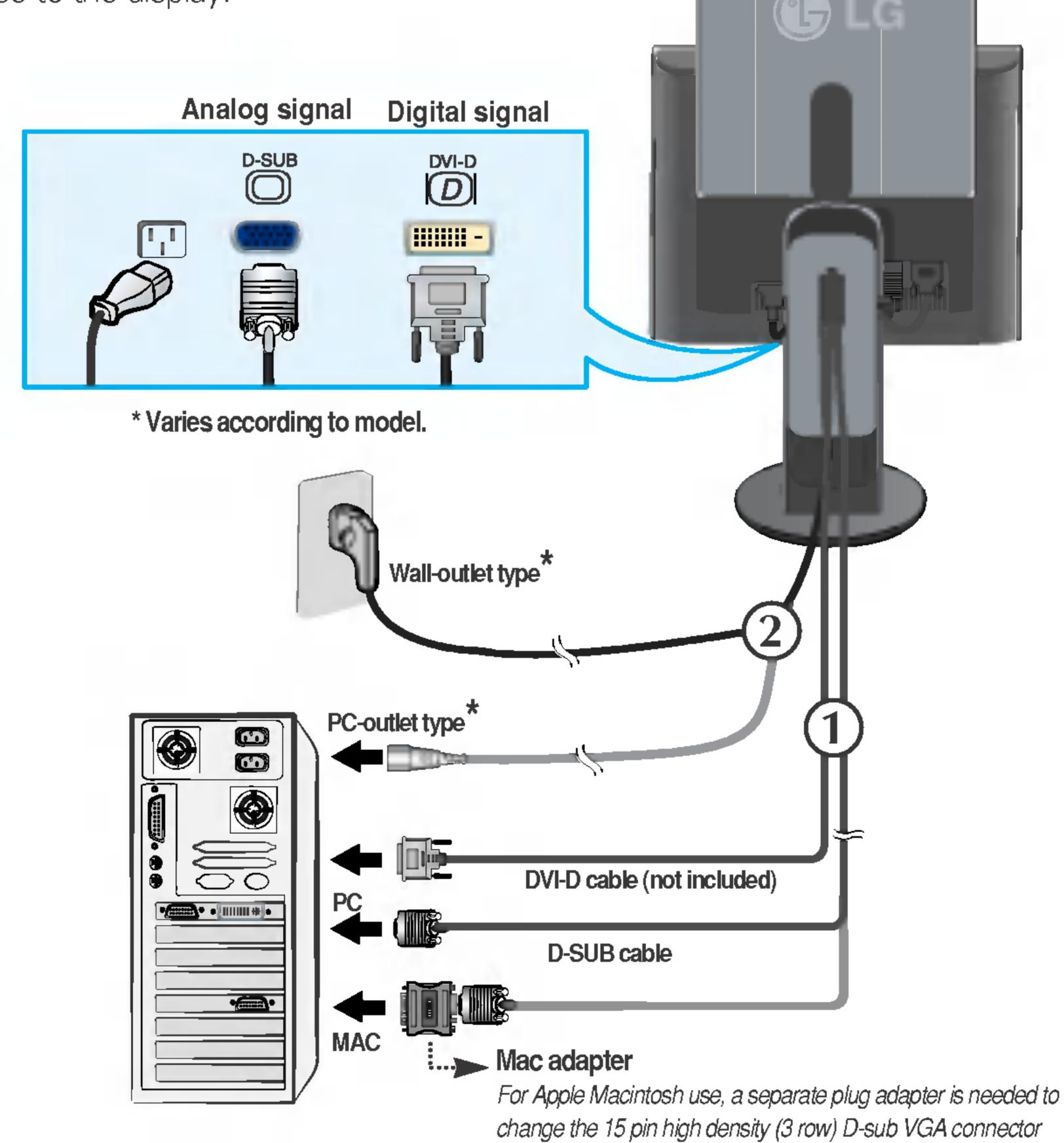
on the supplied cable to a 15 pin 2 row connector.
