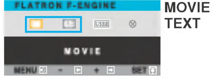
This feature lets you easily select the best desired image condition optimized to the environment (ambient illumination, image types etc).
