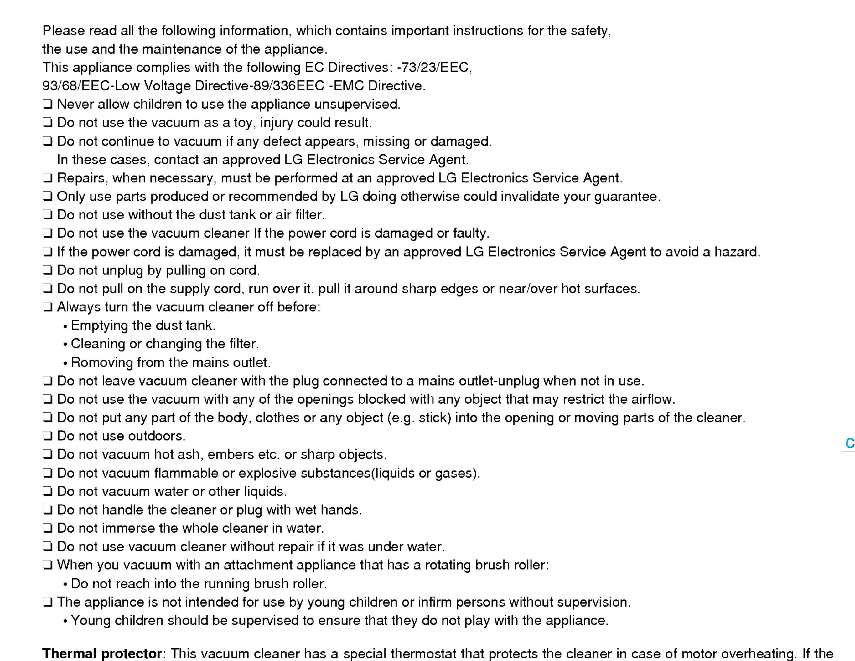
cleaner suddenly shuts off, turn off the switch and unplug the cleaner. Check the cleaner for a possible source of overheating such as a full dust tank, a blocked hose or clogged filter. If these conditions are found, fix them and wait at least 30 minutes before attempting to use the cleaner. After the 30 minutes period, plug the cleaner back in and turn on the switch. If the cleaner still does not run, contact a qualified electrician.
