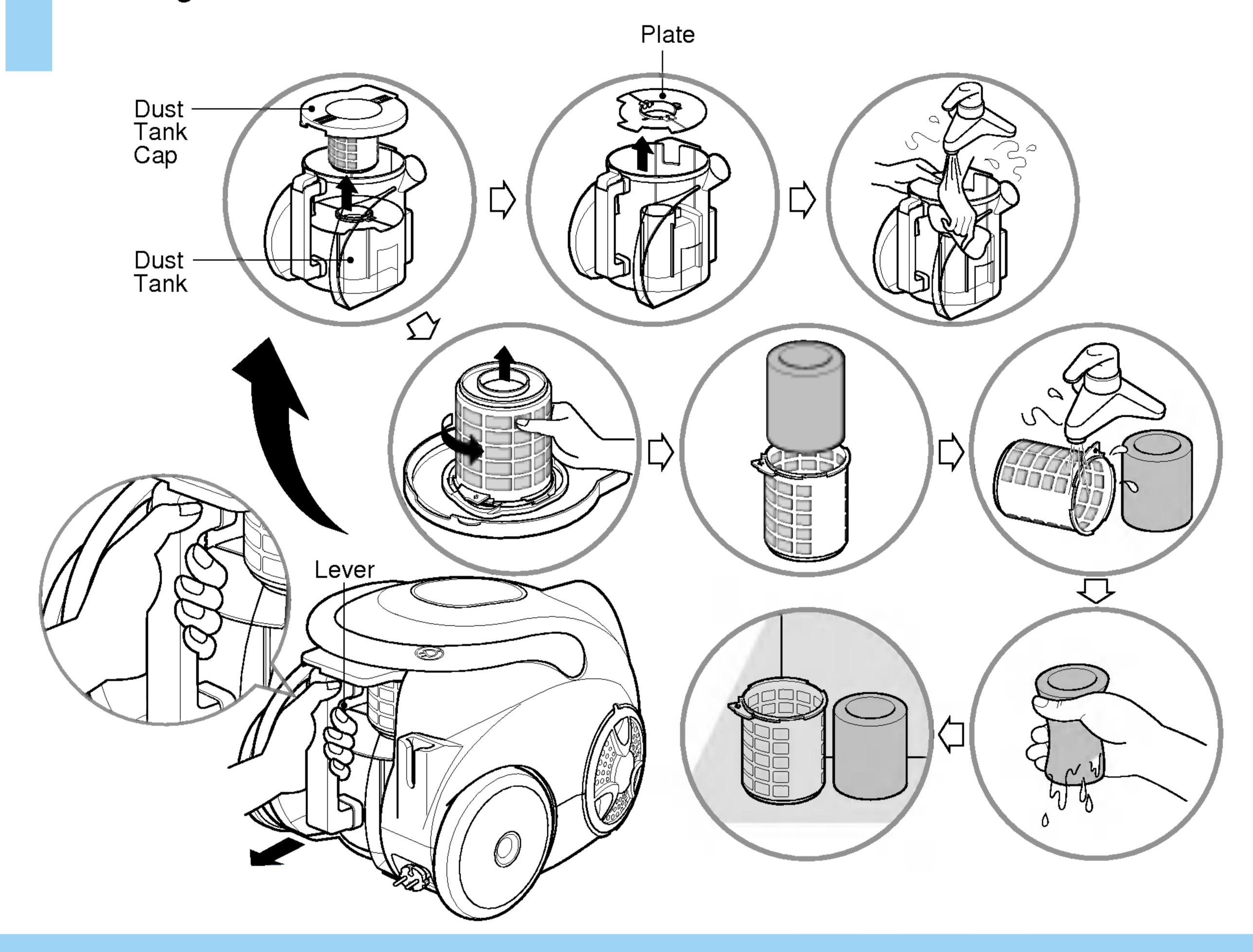
The permanent Air Filter is situated under the dust tank cap. When the indicator light comes on the Air Filter requires cleaning.
