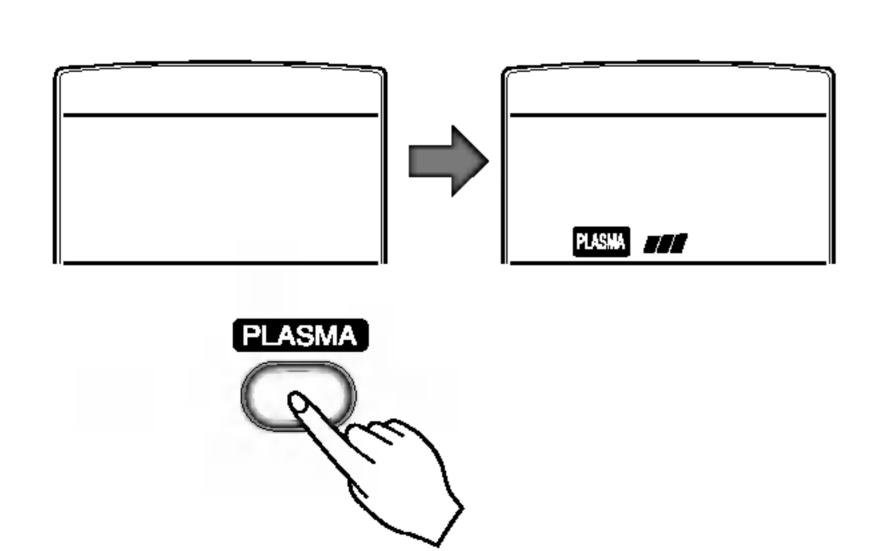
If you press the only NANO PLASMA button, only NANO PLASMA purification function operates.
