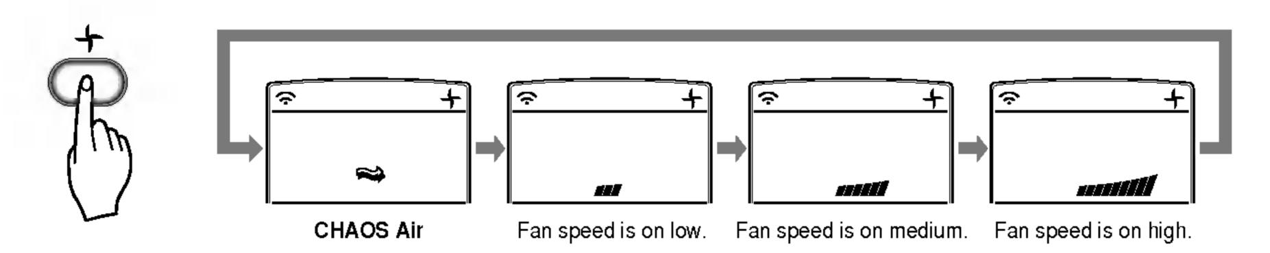
CHAOS Air economizes power consumption and prevents overcooling. The fan speed is automatically changed from high to low or vice versa, depending on the ambient temperature.
