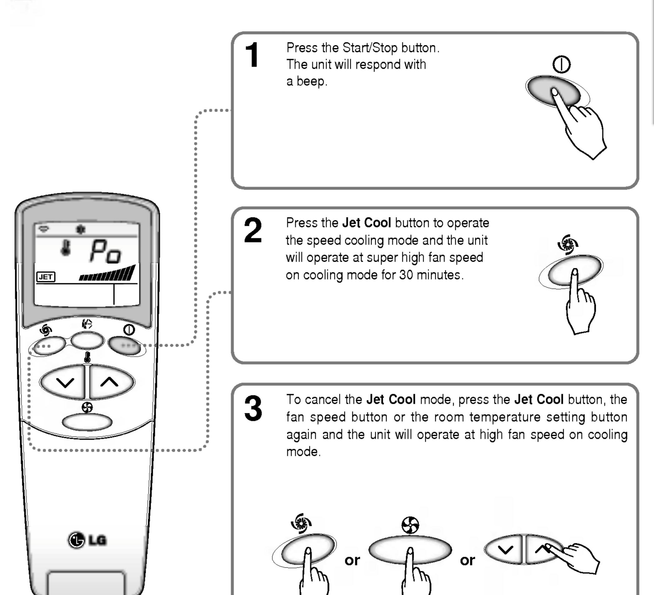
☐ During the JET COOL function at any moment, the A/C starts to blow the cool air at extremely high speed for 30 minutes setting the room temp. automatically to 18°C. It is especially used to cool the room temp. quickly in a hot summer.
