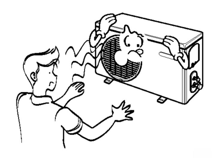
Always inspect gas leakage after the installation and repair of product.
