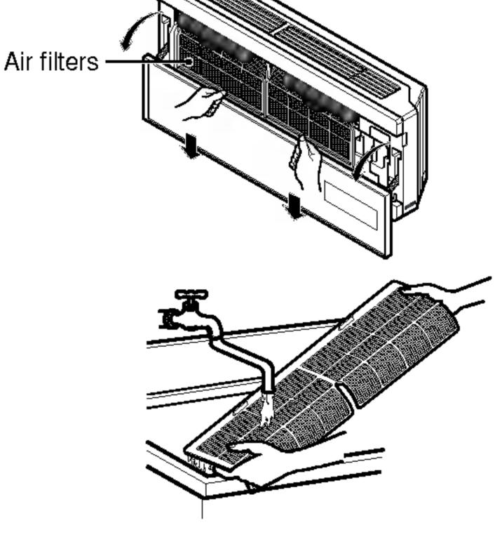
5. Reinstall the air filter dried at the shade and then close the panel.
