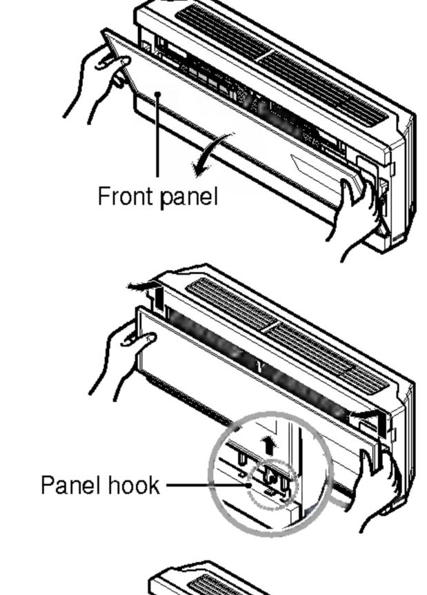
3. Come down the panel and then remove the air filter.
