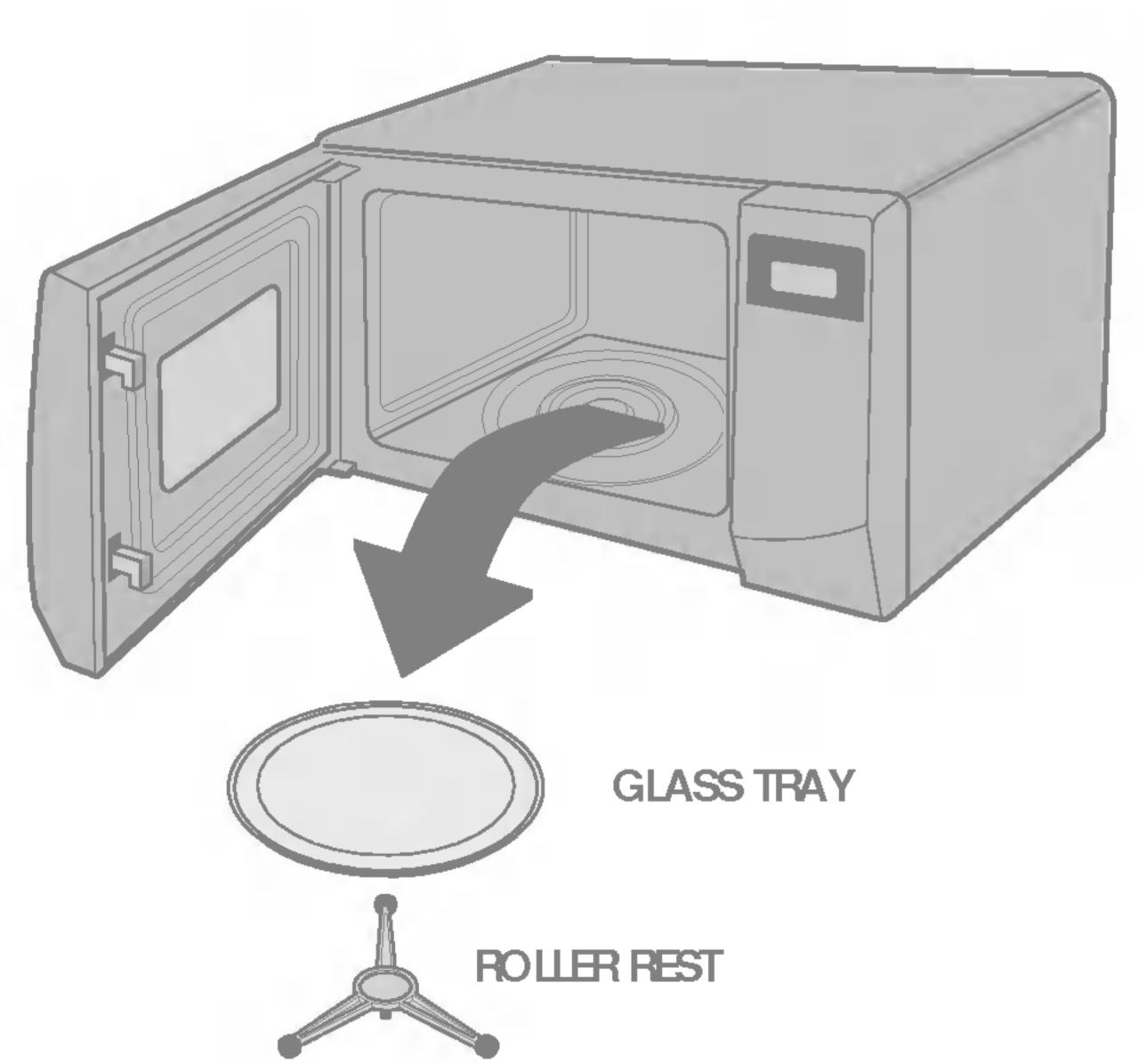
Place the oven in the level location of your choice with more than 85cm height but make sure there is at least 30cm of space on the top and 10cm at the rear for proper ventilation. The front of the oven should be at least 8cm from the edge of the surface to prevent tipping.
