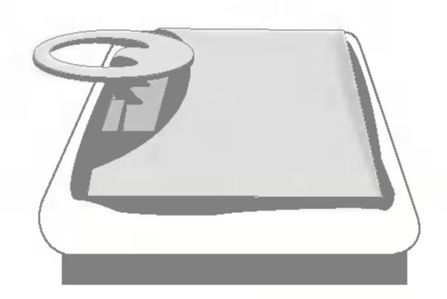
2. Hold down the release button inside the stand and strongly pull out the stand with your two hands.
