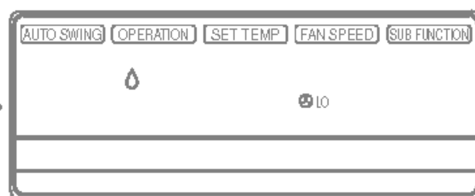
Soft Dry Operation
