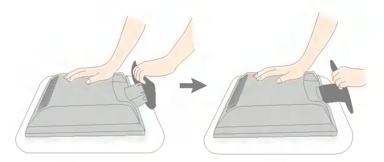
3. Place the monitor upright and adjust the angle of the stand base as desired. Adjust the stand base angle with two hands, holding the monitor head.
