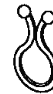
Tie Holder (option) - Arrange the wires with the tie Holder.
