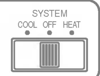
Move the system switch to the "OFF" position in order to stop heating operation.
