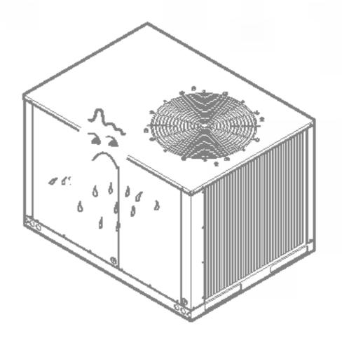
Condensation occurs when the airflow from the air conditioner cools the warm air.
