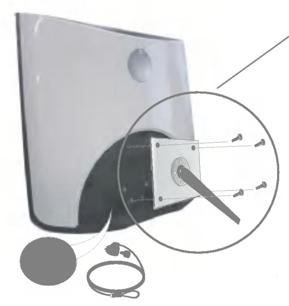
VESA wall mounting Connected to another object (stand type and wall-mounted type. This monitor accepts a VESA-compliant mounting interface pad.-optional) For further information, refer to the VESA Wall Mounting Instruction Guide.
