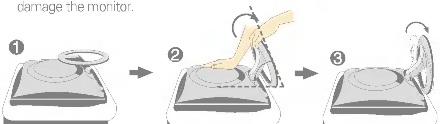
4. Place the monitor upright and adjust the stand base angle as desired. Adjust the stand base angle holding the monitor head part with both hands.
