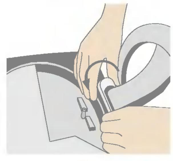
2. Slide off the lower section of the cover base with two hands as shown in the picture.
