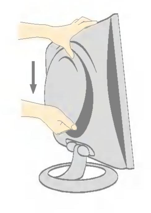
1. Separate the back cap by sliding its lower section downward as shown in the picture.
