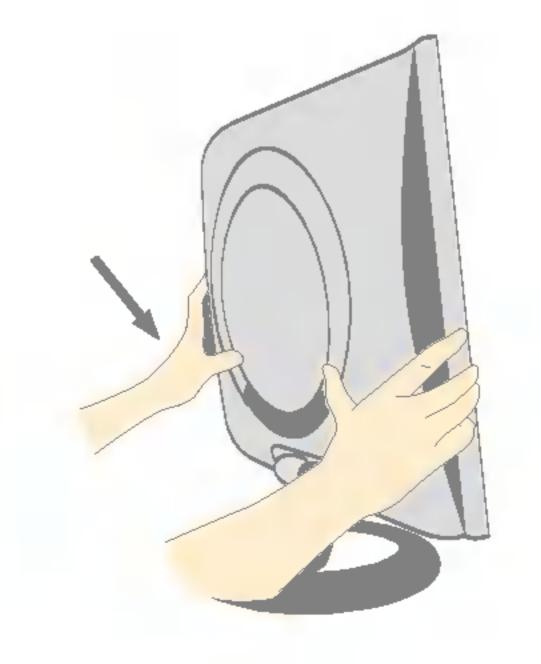
4. Insert the back cap along the bottom grooves on both sides, holding the bottom.
