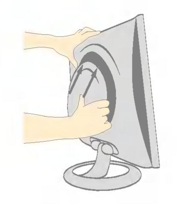
3. After the cables are connected, set the back cap into the groove of the upper section and reassemble by pushing upward.
