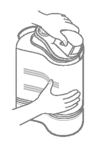
Fix the connecting part in place by means of the holder ring as shown.
