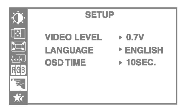
VIDEO LEVEL This item is used to select the monitor's input signal level. The normal level used for most PCs is 0.7V.
