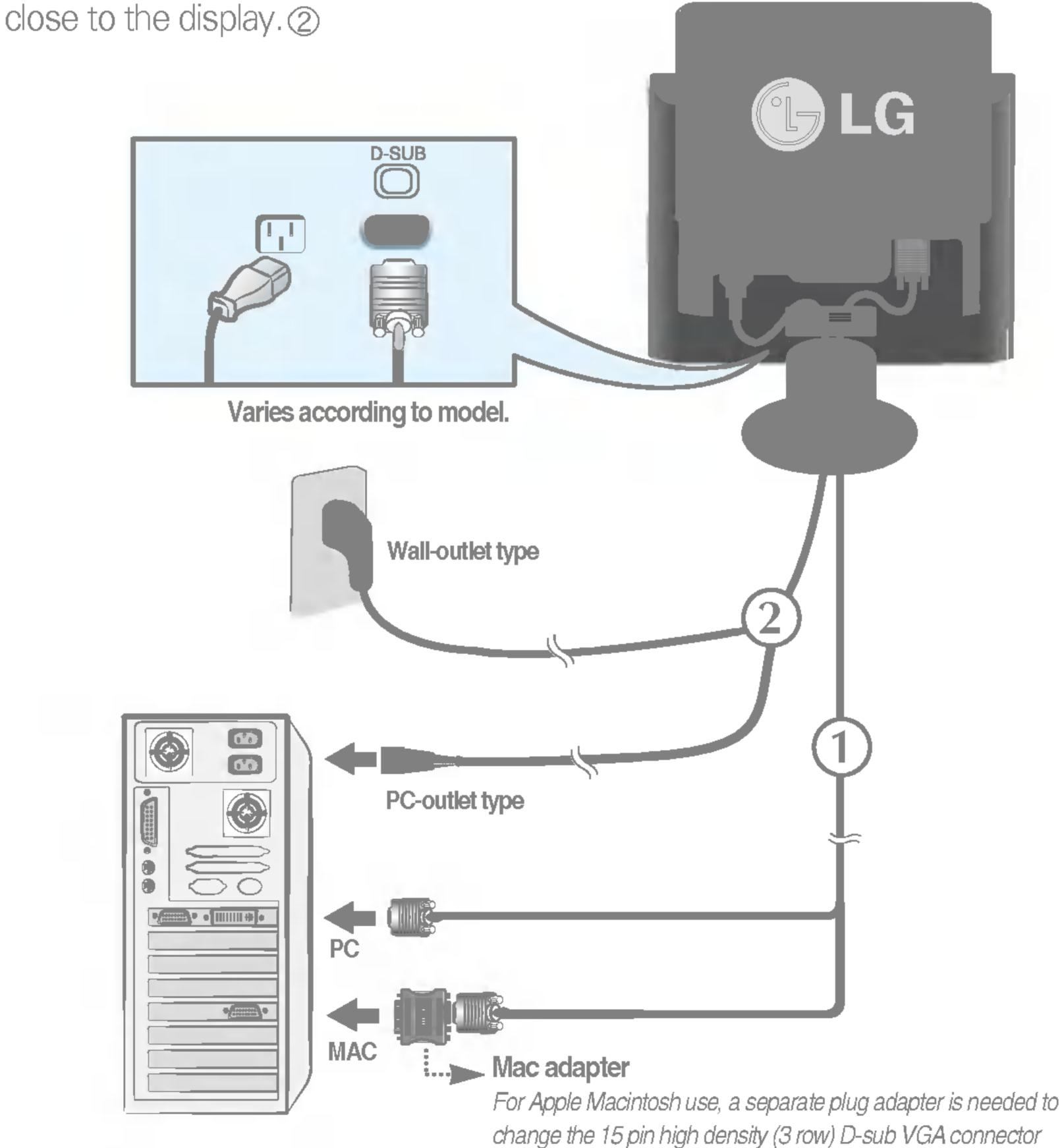
on the supplied cable to a 15 pin 2 row connector.
