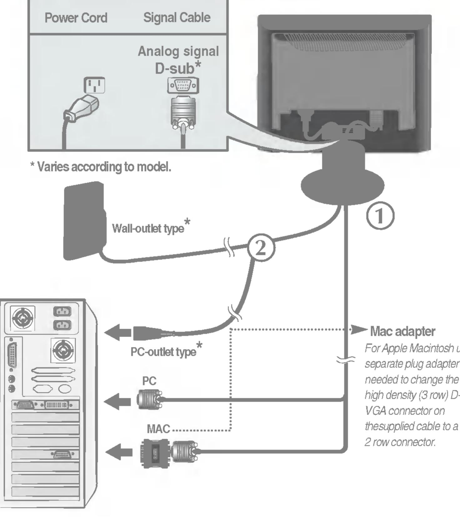
For Apple Macintosh use, a separate plug adapter is needed to change the 15 pin high density (3 row) D-sub thesupplied cable to a 15 pin
