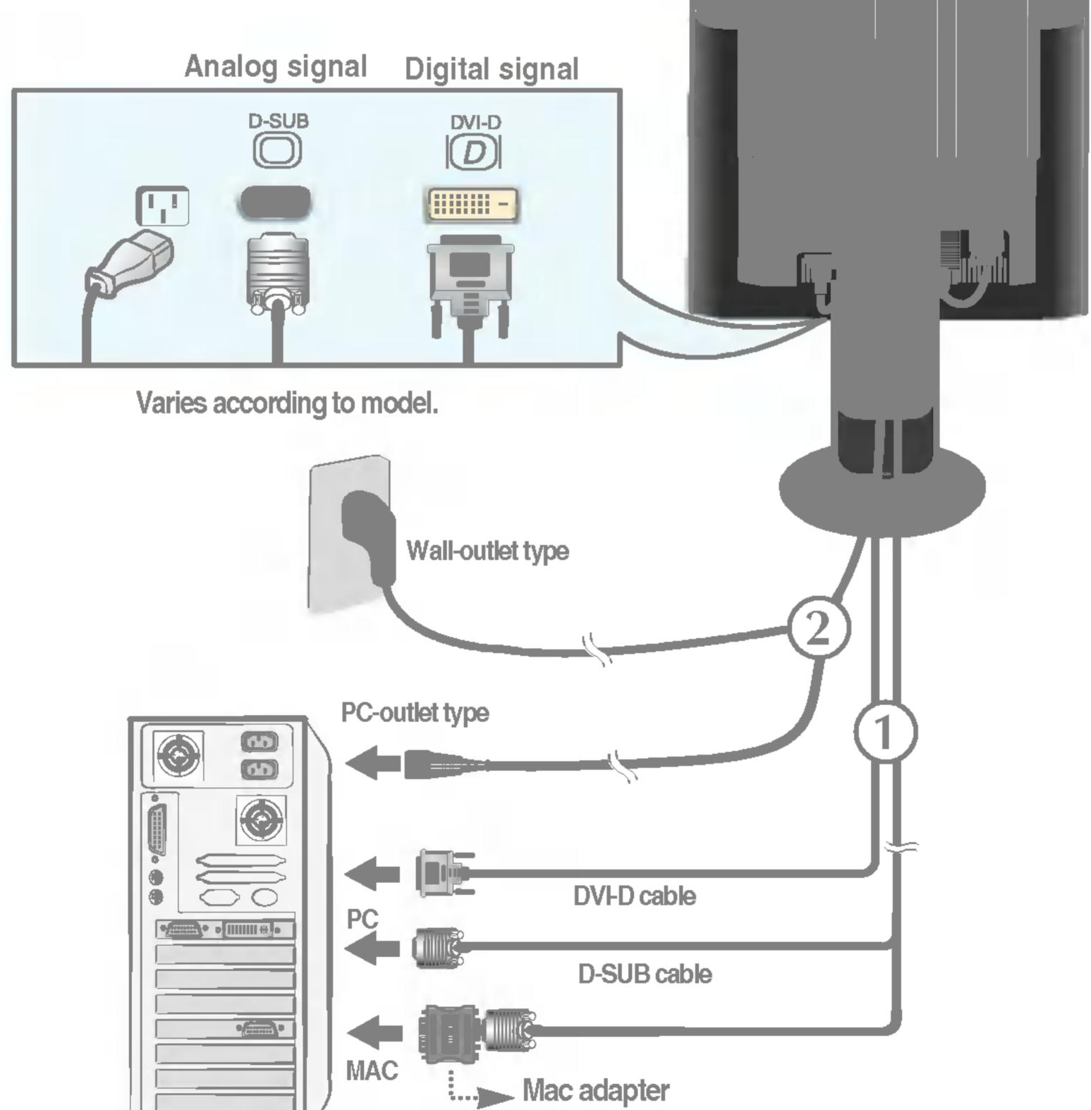
For Apple Macintosh use, a separate plug adapter is needed to change the 15 pin high density (3 row) D-sub VGA connector on the supplied cable to a 15 pin 2 row connector.
