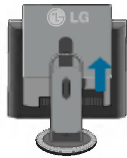
2. Please the monitor on a piece of cloth or other soft surface with the front side facing downward. **3.** Separate the stand base using a screwdriver as shown in the picture.
