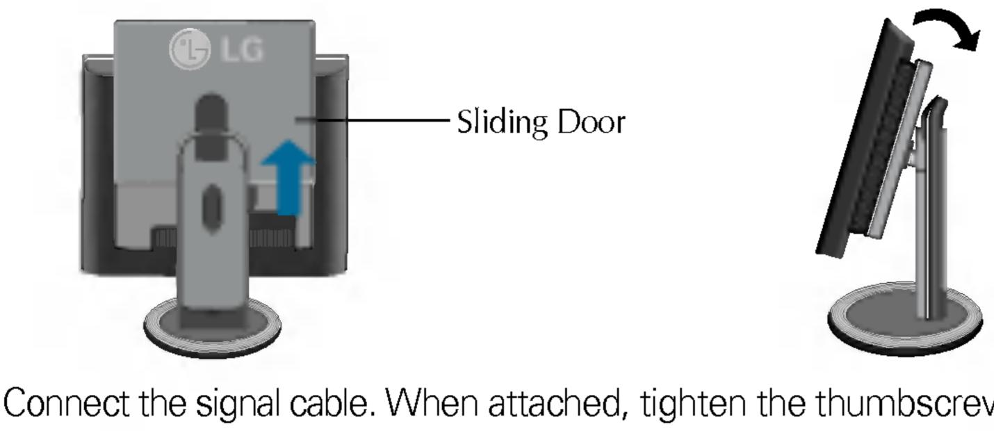
Connect the signal cable. When attached, tighten the thumbscrews to secure the connection.
