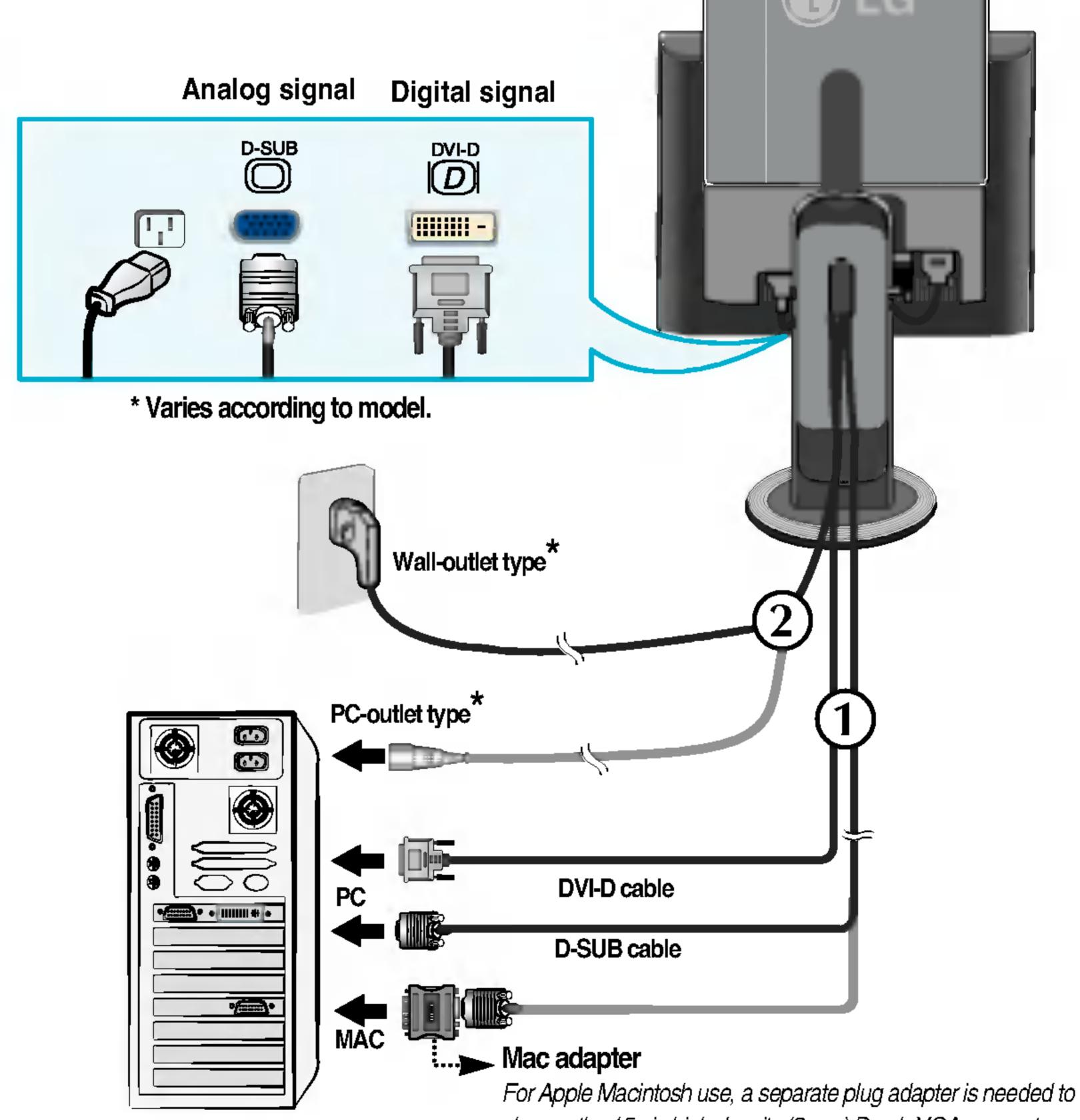
For Apple Macintosh use, a separate plug adapter is needed to change the 15 pin high density (3 row) D-sub VGA connector on the supplied cable to a 15 pin 2 row connector.
