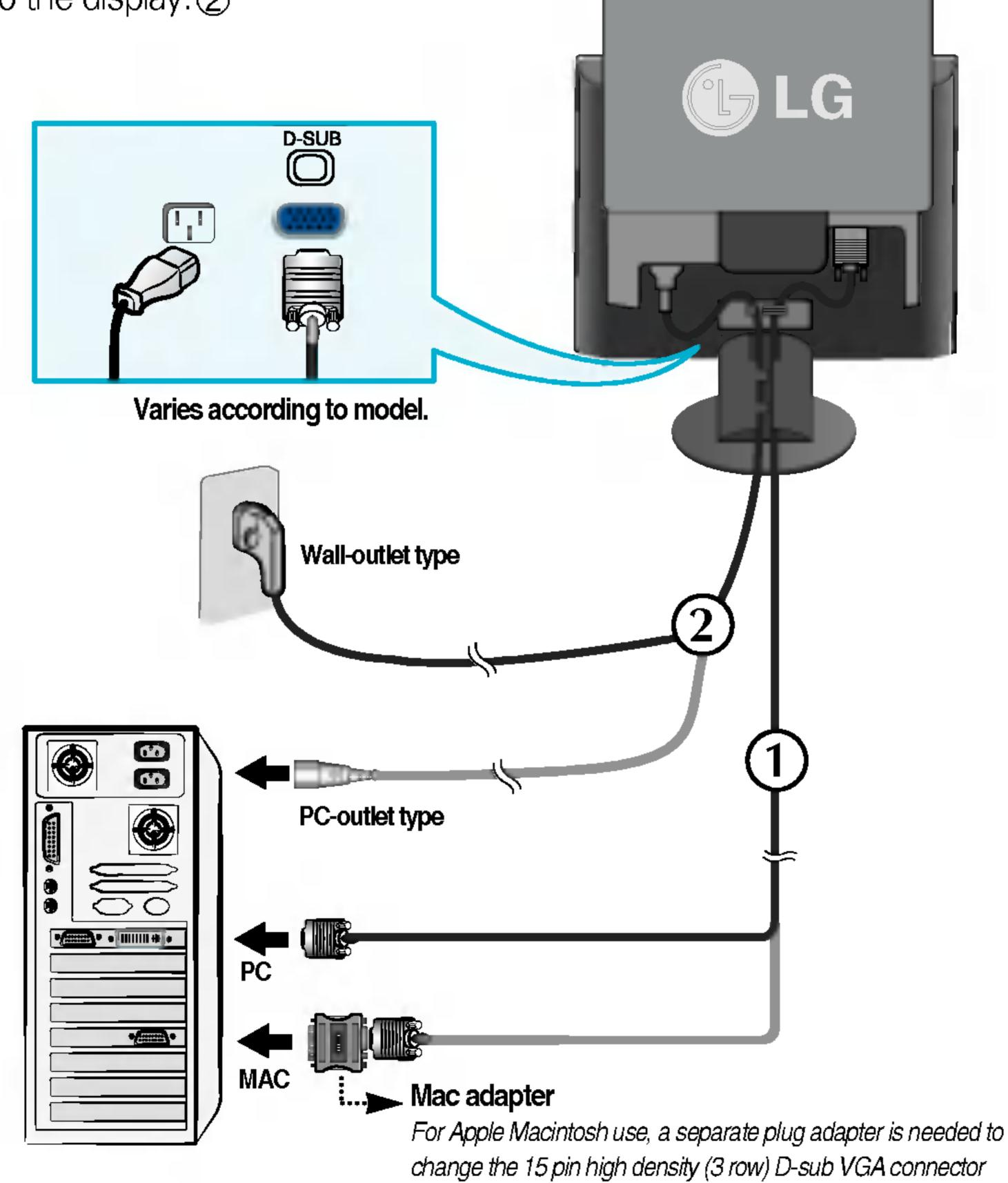
on the supplied cable to a 15 pin 2 row connector.
